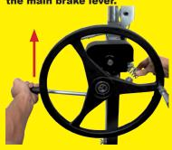
Pull the steering wheel to remove it from the axis. Be careful not to lose the axis pin pulling the steering wheel.
