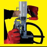
Fix the arms with the two 43 mm (1<sup>3/4</sup>") screws and nuts, using a 13 mm (1/2") flat wrench and a 6 mm (1/4") hex wrench. Make the arms marks match:
