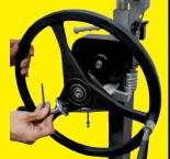
Remove the spring lifting completely up the main brake lever.
