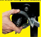
Replace the steering wheel on the main axis ensuring that the pin takes place in its location in the steering wheel.
