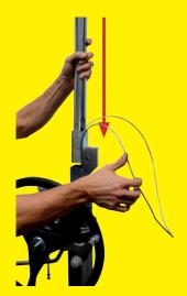
Put the axis maintaining the pulley back and tighten the nut on the axis with a 17 mm (11/16") flat wrench and an 8 mm (5/16") hex wrench.
