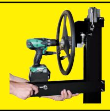
Insert the hex bit fixed on the power drill in the hex hole located in the middle of the steering wheel. Turn the power drill to block it against the power drill support base. Set the power drill on "maximum torque", rotating on clockwise direction.
