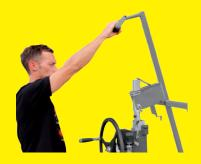
Block the 2 wheel brakes and load the board.
