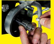
Pull the brake lining to remove it from its location.
