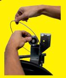
Unscrew the nut from the axis that maintain the cable at the mast pipe. Use a 10 mm (3/8") flat wrench and a 5 mm (3/16") hex wrench.
