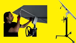
Turn the steering wheel while pressing the main brake lever to lift the board until the ceiling.
