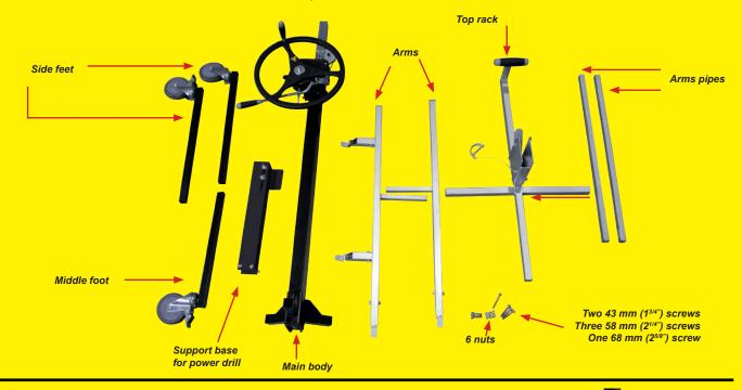
Fix the side and middle feet on the fixing plate of the main body with three 58 mm (21/4") screws and nuts. Use a 13 mm (1/2") flat wrench and a 6 mm (1/4") hex wrench. Position the side foot with brake on the same side than the main and safety brake
